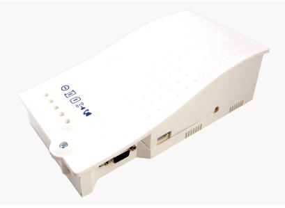
The Digital Communication Platform (DCP) provides an information gateway between all compatible connected devices in the lift shaft and our cloud based monitoring platform; the Avire Hub.
